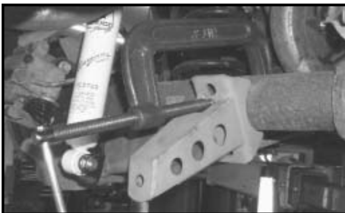
Figure 4b.0 - Assemble driver side Axle Tower.
