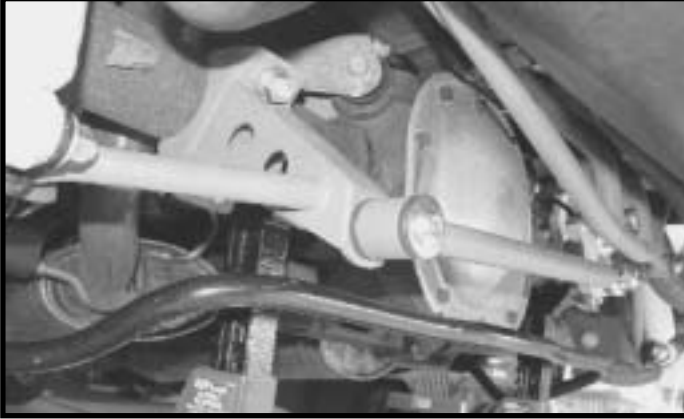
Figure A - Watts installed. View from driver/rear.
