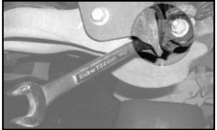
Figure 2.0 - Remove rear lower shock mount from axle..
