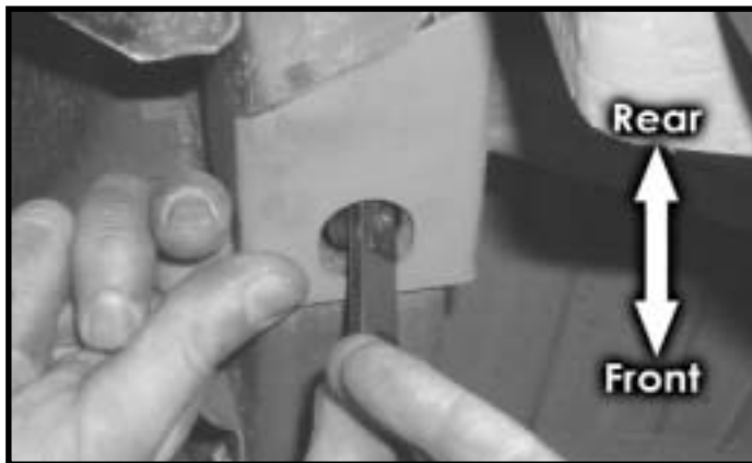
Figure 3a.4 - Insert tapping plate.
