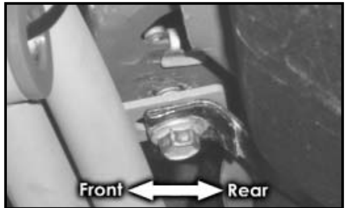
Figure 3a.2 - Sandwich Watts Cradle tabs.
