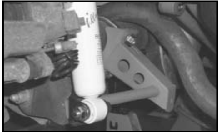
Figure 4a.0 - Assemble driver side Axle Tower.
