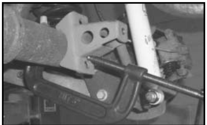
Figure 4b.1 - Assemble passenger side Axle Tower.
