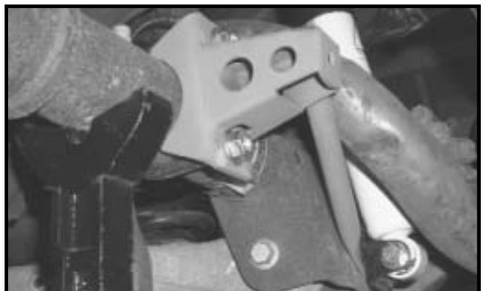
Figure 4a.1 - Assemble passenger side Axle Tower.
