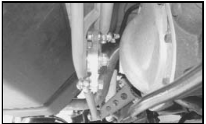
Figure D - Watts Installed. Side view from passenger side.
