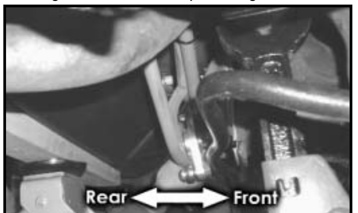
Figure 2.6 - Orient Watts Cradle assembly.
