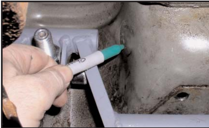
Figure 3.7 - Mark transmission tunnel.
