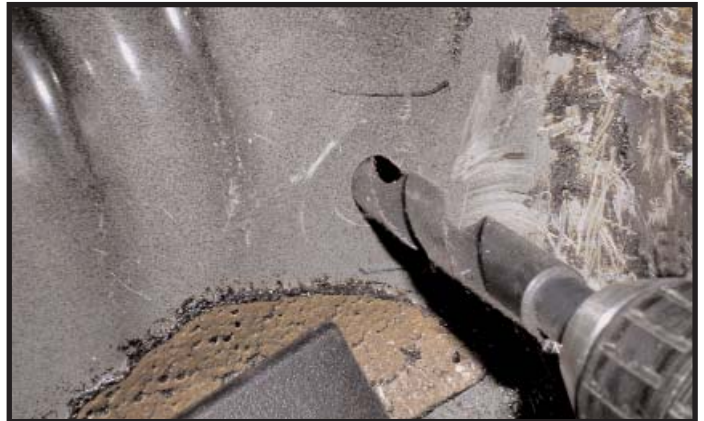
Figure 3.8 - Drill hole thru transmission tunnel.
