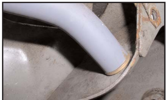
Figure 3.3 - Fit washers/sleeves for cradle mount at UCA.
