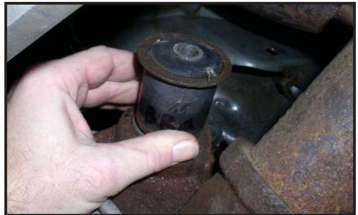
Figure 1.4 - Remove UCA bushings from rear axle.
