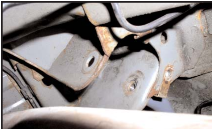
Figure 3.1 - Drill out UCA mounting holes.
