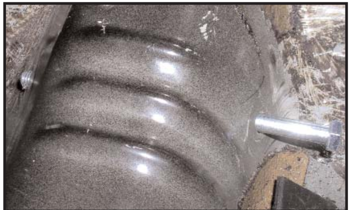
Figure 3.9 - Push thru-bolt through transmission tunnel.
