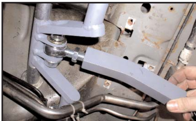
Figure 4.1 - Thread link onto front rod end.
