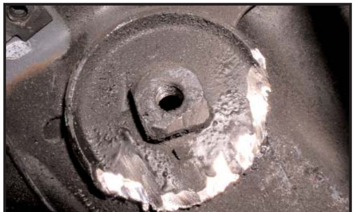
Figure 3.6 - Eliminate Front Cradle interference.
