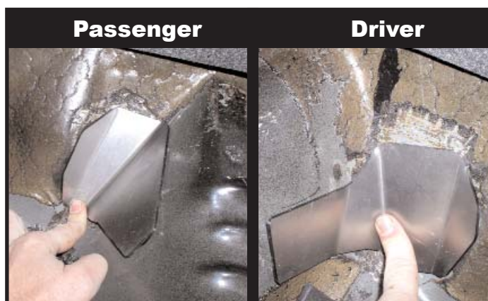
Figure 3.11 - Position floor reinforcement plates.
