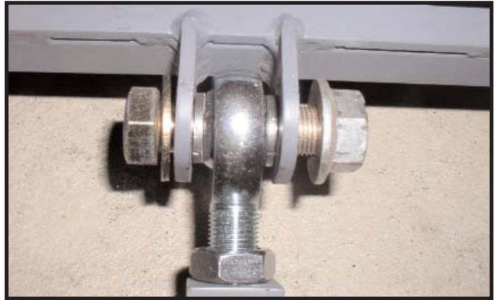
Figure 4.3 - Install rod end bolt and spacers.
