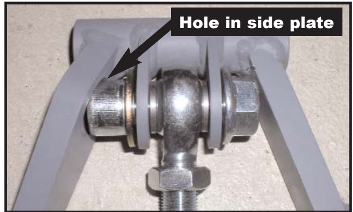
Figure 3.0 - Install rod end on front cradle.
