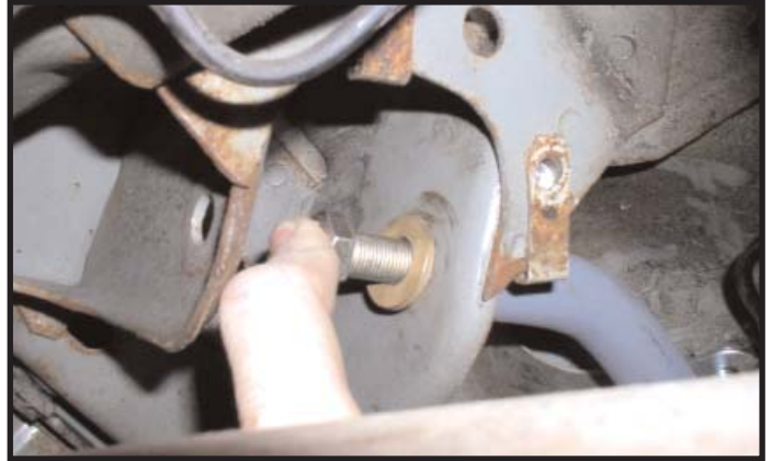
Figure 3.4 - Install UCA fasteners.
