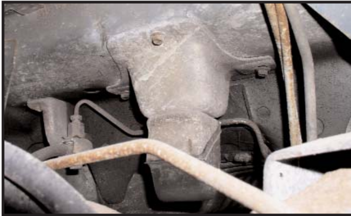
Figure 1.2 - Remove pinion snubber and bracket.
