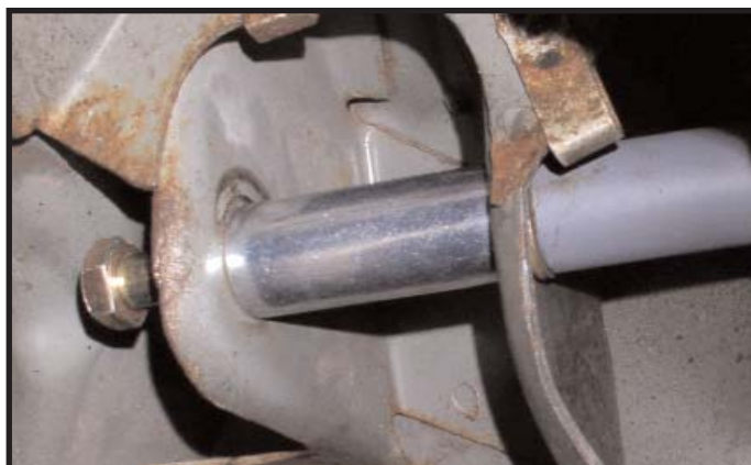
Figure 3.17 - Double shear spacer installation.
