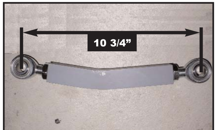
Figure 4.2 - Link length reference diagram.
