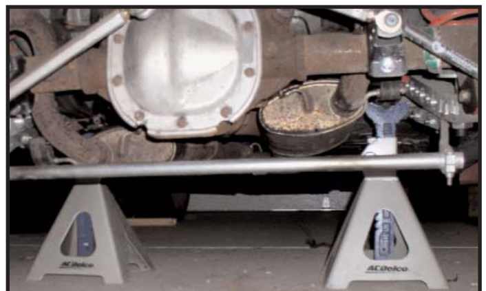
Figure 1.1 - Support vehicle at LCA forward mount.
