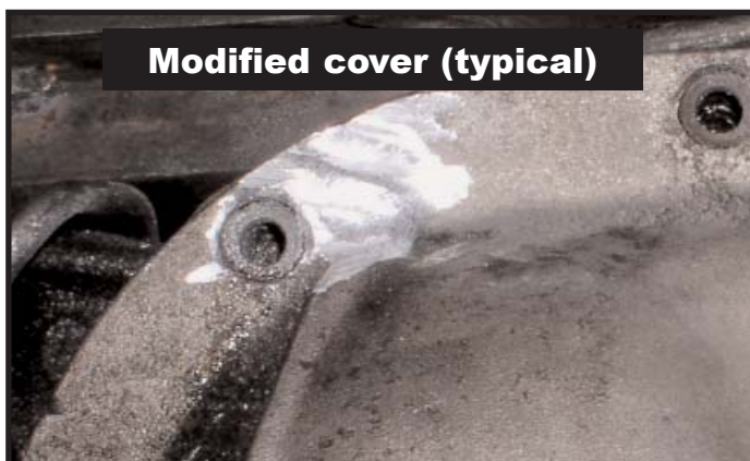
Figure 2.5 - Remove material from axle cover.
