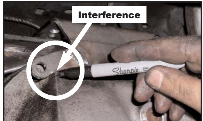
Figure 2.4 - Mark cover for material removal.
